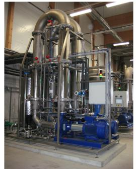
Ultrafiltration with ceramic Multibore tubular membranes
