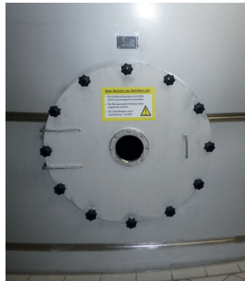
Manhole with sight glass
